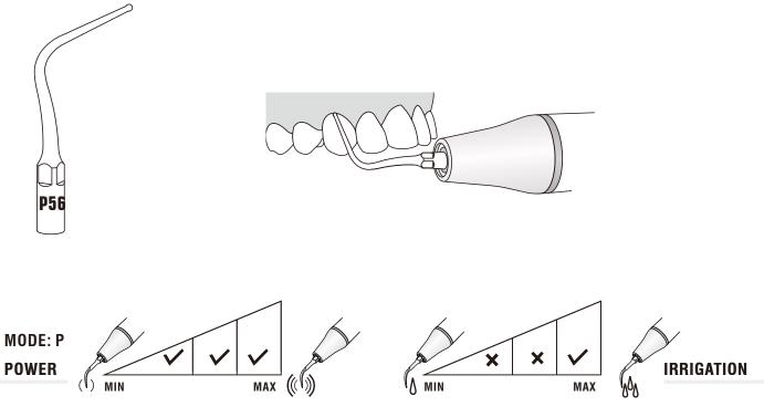
Water volume control: Ensure that the cooling water reaches the end of the tip. Function: For the treatment of root bifurcation, removal of supragingival large calculus and plaque.
