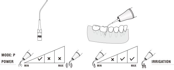
Volume of water: Ensure the cooling water reach the end of the tip Functional Description: Used for gingival large stones and dental plaque Applicable area: All teeth buccal and lingual site of dental implant or prosthesis. Operation method: The tip is parallel to the long axis of the tooth.and ensure the 2 mm right or left tip niddle site adapt the tooth surface. Move the tip front and back. Warn: Please ensure that there is water coming out from the handpiece to avoid damage to the tip
