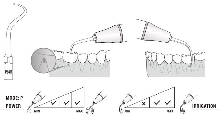
Volume of water: Ensure the cooling water reach the end of the tip Functional Description: Used for gingival large stones and dental plaque Applicable area: All teeth buccal and lingual site. Operation method:The tip is parallel to the long axis of the tooth. and ensure the 2 mm right or left tip niddle site adapt the tooth surface. Move the tip front and back.
