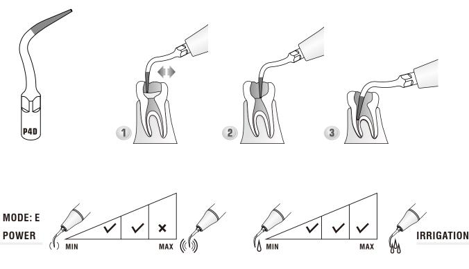
**E6**(ED6) Thin and flexible, used for removing foreign body in deep canal.
