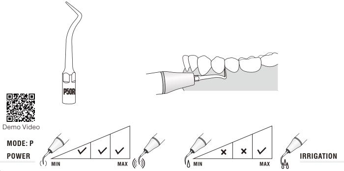
Volume of water: Ensure the cooling water reach the end of the tip
